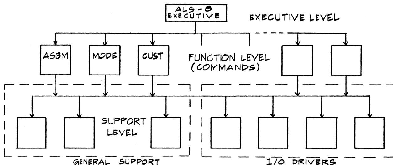
The top level, the executive level in this diagram, represents the control center. It is this section which controls the communications with the terminal, decides which function is to be executed, and reports on errors to the user. Each block on the function level corresponds to a command from the ALS-8 command set. These routines, for efficiency's sake, make heavy
